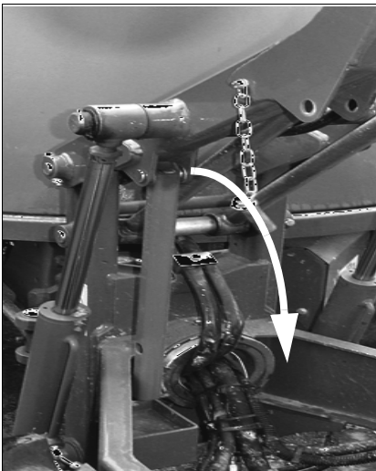
Fig. 1: High-tip dump bucket maintenance strut
