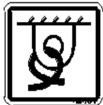
Fig. 7: Label for points used for strapping down the machine
