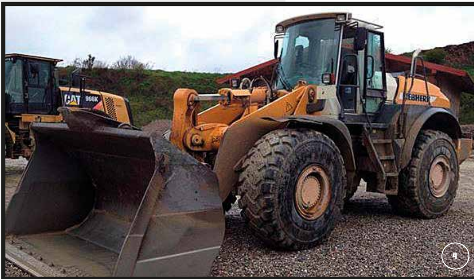
4. The L580 was a third generation machine and the flagship loader for Liebherr in the early 2000s. At the time it was the largest hydrostatic drive wheel loader in the world. It was used extensively in quarry, gravel and even forestry operations.
