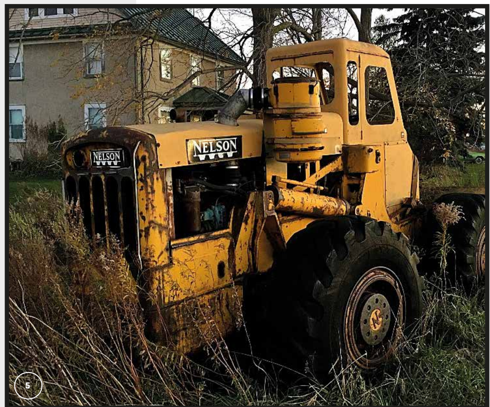
5. Not a very well known loader manufacturer, Nelson produced a small range of wheel loaders beginning in 1957. The model 250 illustrated had a 2½ cubic yard bucket and was powered by a GM 4-53 diesel. Gasoline engines could also be specified.
