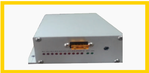
Tilt rotator control system (24 V, 12 V)
